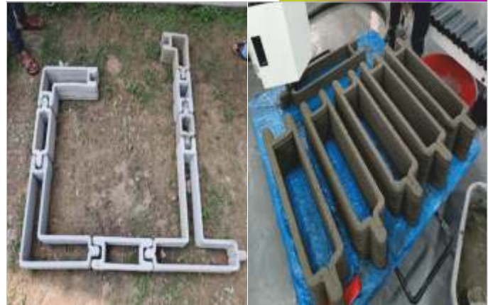
Figure : 3D printed SCBA/fly ash based interlocking block units and printing of hollow 3DPCB units
