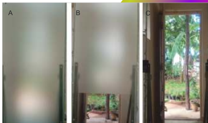
(A) Opaque State, (B) Curtain effect to bring the transparency in the selected area, (C) complete curtain raise to bring full transparency
