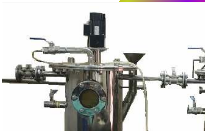
Figure: Laboratory scale anaerobic reactor - 45 litre capacity
