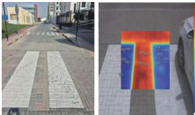
Figure: Outdoor field demonstration of radiative cooling coating showing significant surface temperature reduction under direct sunlight, confirmed by infrared thermography
