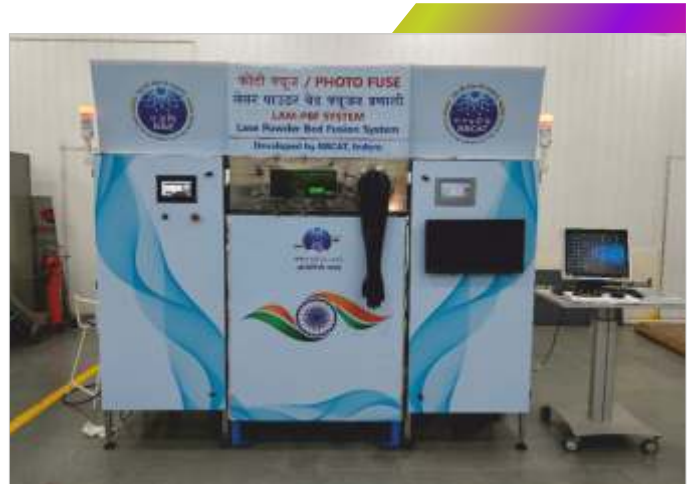
Laser Additive Manufacturing System using Powder Bed Fusion System
