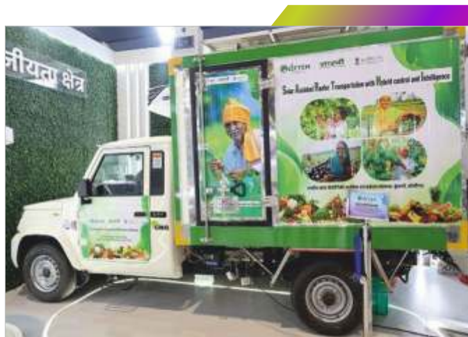
Solar Assisted Reefer Transportation with Hybrid control and intelligence (SARTHI)
