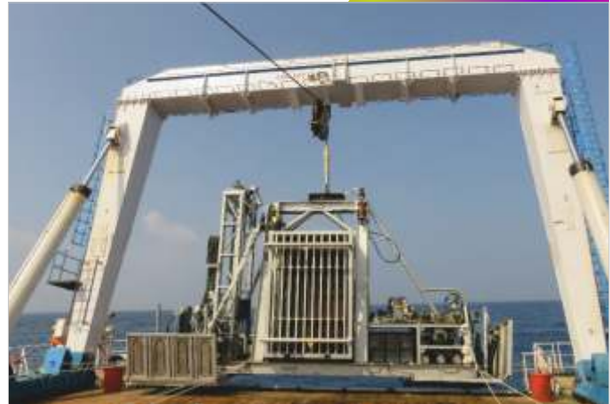
Autonomous Coring System Onboard Ship
